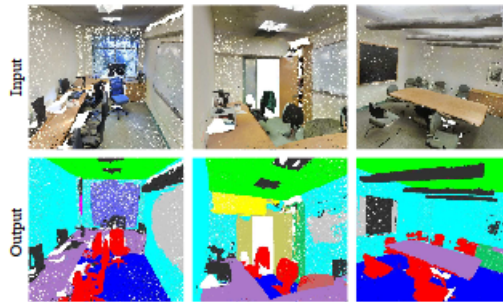
Figure 8: Examples of PointNet’s segmentation network applied to pointclouds of indoor office rooms, from one scan the model is able to identify multiple features within the scene (i.e. Chairs, Walls, etc.) with a good level of accuracy, all while keeping the data purely 3D. Figure taken from [20]
