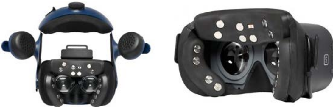
Figure 2.1: emteqPRO mounts for the HTC Vive Pro (left) and Pico G2 4K (right) [20].
