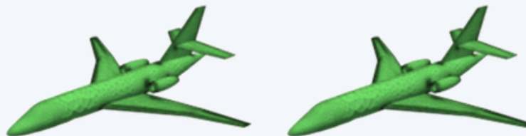
Figure 1 : Falcon: Target (left) and predicted (right) anisotropic meshes for a transonic flow condition
